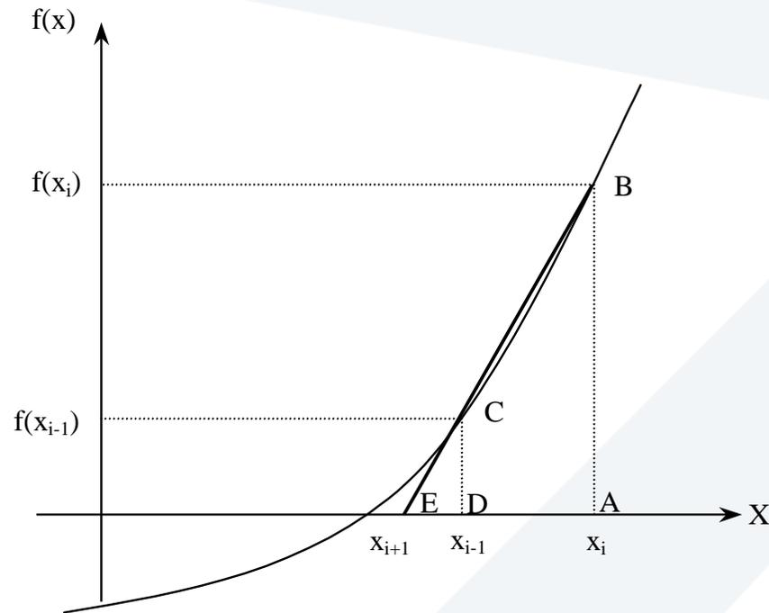
Figure 2 Geometrical representation of the Secant method.
